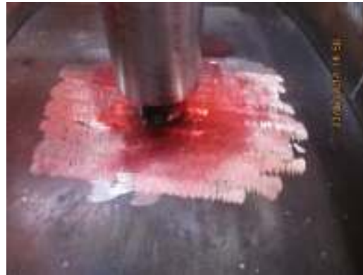
3) Weld all round the tip of TD. Check with non destructive penetration test for good welding.
